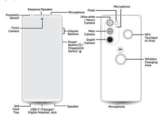
**Use a digital headset:** To use a digital headset, you'll need one with a USB-C connector. If using a 3.5mm digital headset, you'll need an adapter to connect a 3.5mm connector to USB-C. Digital headset may be sold separately.
