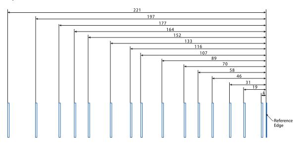
Rib pattern for Lexmark C4150, CS720, CS725, CS727, CS728, CX725, CX727, XC4140, XC4150
