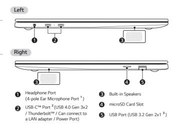
1 The 4-pole ear microphone port supports US 4-pole standards, but not the European 4-pole ear microphone.
