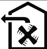
The air must not be discharged into a flue that is used for exhausting fumes from appliances burning gas or other fuels (not applicable to appliances that only discharge the air back into the room).
