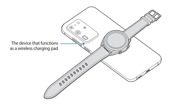
2 After fully charging, disconnect the Galaxy Watch3 from the device that functions as a wireless charging pad.
